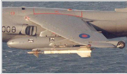
Sea Harrier FRS Mk 1 wing details including air-to-air Sidewinder missiles
